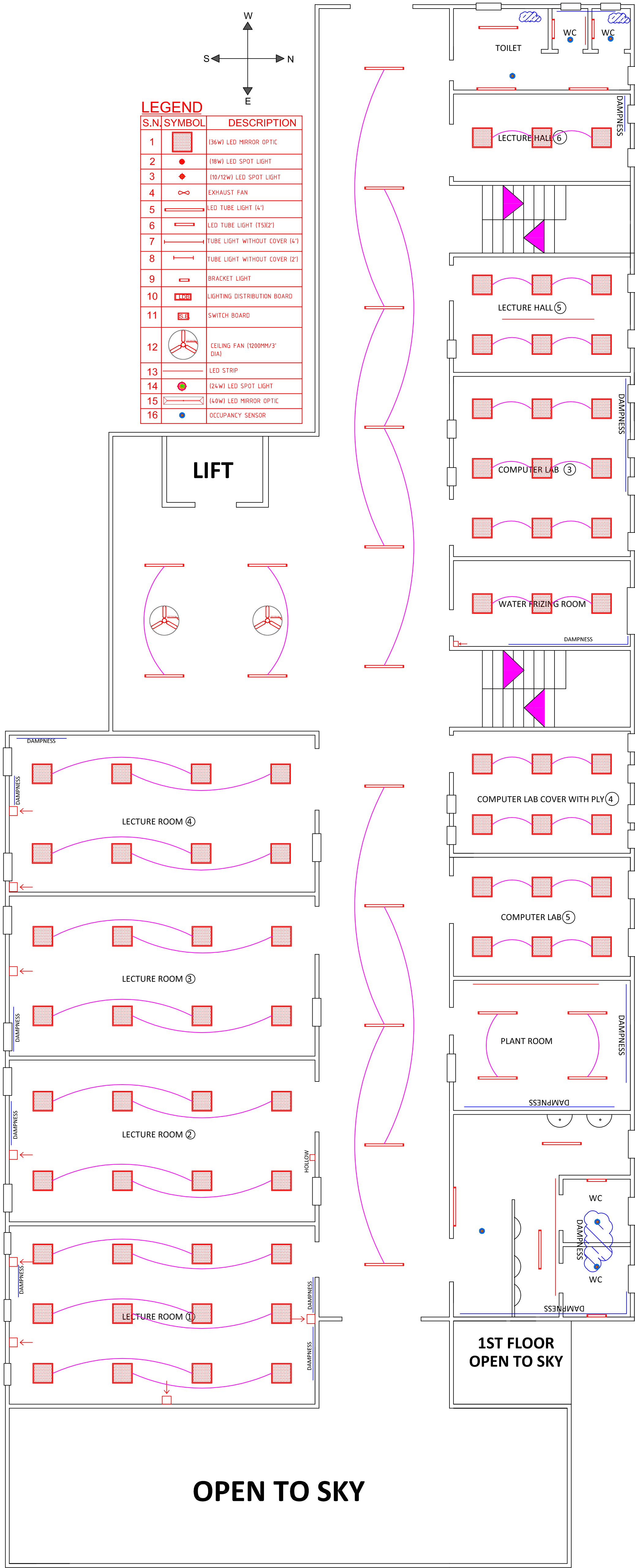
2ND FLOOR REFLECTED CEILING PLAN WITH LOOP
